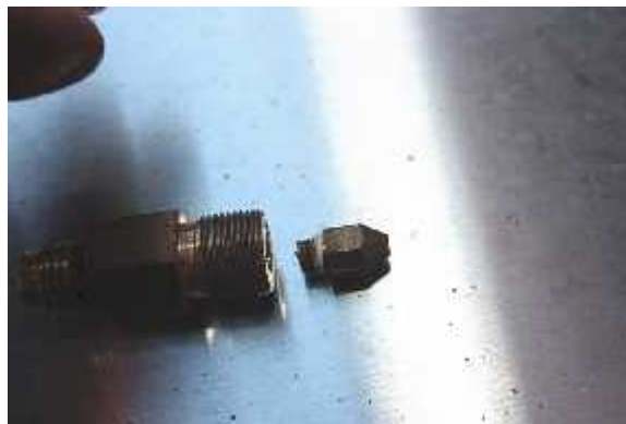
Infrared burner orifice
