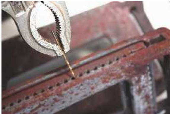
Use 1/16 drill bit to ream gas port
