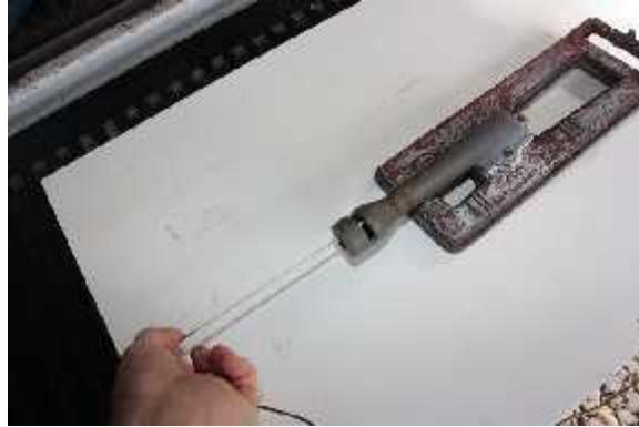
Swab venturi with venturi brush or wire coat hanger.
