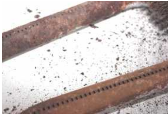
This is a Ducane S Burner, from a 15 year-old model, which shows the rusted part. The electrode needs replacing, but the burner still has a year or so of life left.
