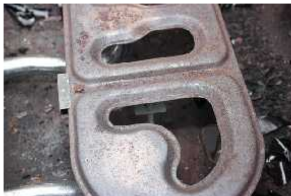
This is from a Great Outdoors DG450. This burner hasn't had much use. Note the two bolts holding it to the grill bottom. You will probably have to grind off the bolt heads to get the burner out when it needs replacing.
