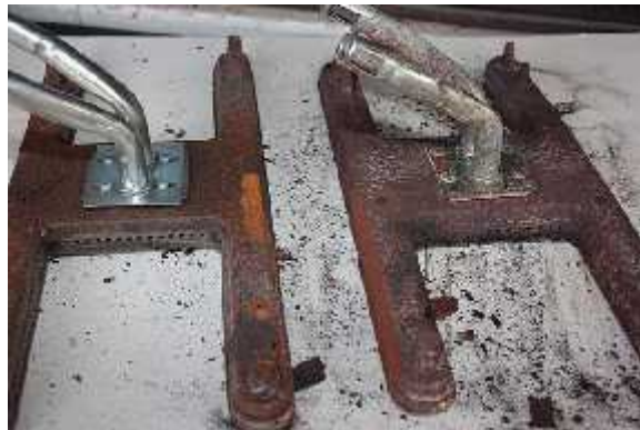
Great Outdoors 1000 cast iron burners. The right one needs the gas ports cleaned and blown out there as well as through the venturi openings.
