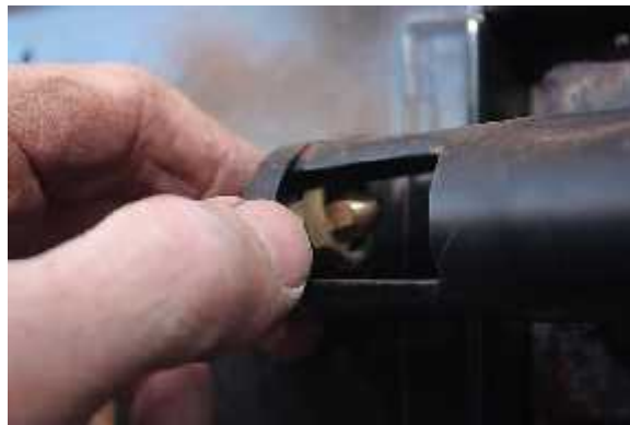
Remove nut holding the fitting - DO NOT DROP!!! Or LOSE!!!
