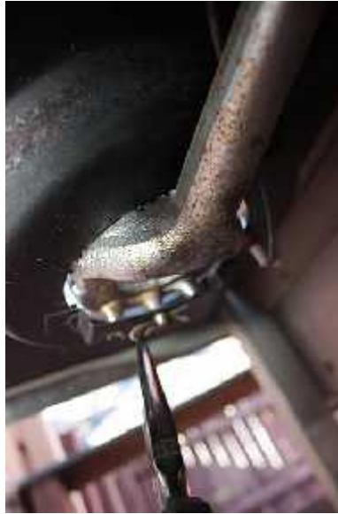
Remove cotter pin holding side burner under shelf.
