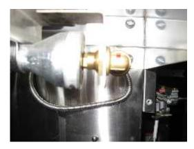
The orifice for the side burner is under the side burner shelf in front of the burner venturi. It will have to be removed carefully with wrenches to allow drilling.
