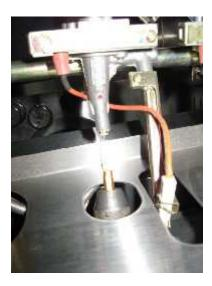
After loosening the front panel and removing the main burners you can drill the valve orifices with a drill in a manual holder through the front burner opening in the grill. <u>DO NOT USE</u> an electric drill. The drill bit will break.
