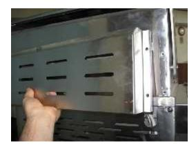
To get to the rotisserie burner you'll have to remove screws on the back of the grill and inside the grill that hold the rotisserie burner in place. You will have to remove the orifice from the burner in order to get the drill bit in place.
