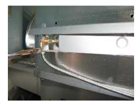
Use some wrenches to loosen and remove the rotisserie burner orifice to drill out with a 10000BTU #54 drill bit for Natural Gas.
